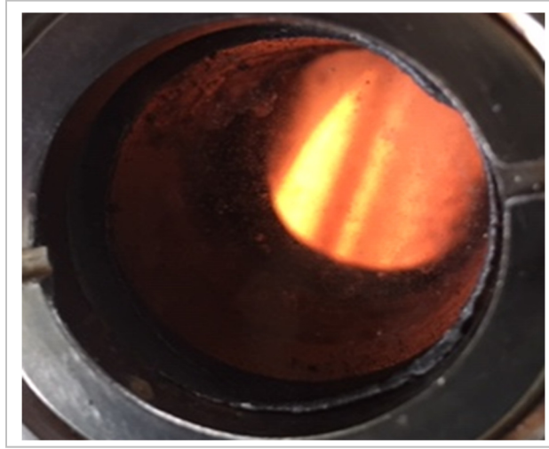
Fig.24. Soot origination in oxy-hydrogen-methane flame at decreasing \text{H}_2 flow [6 l/min]
