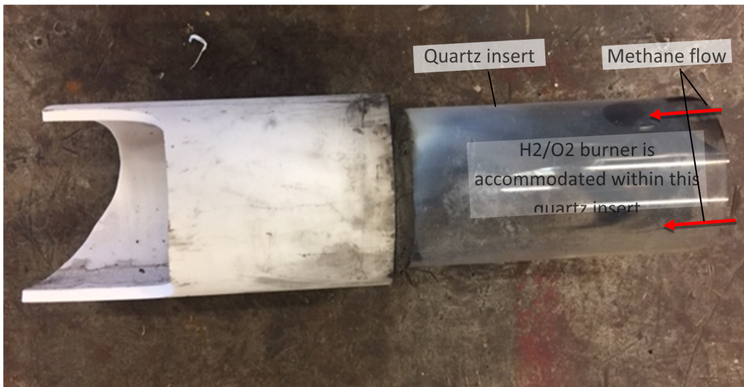
Fig 16. The broken internal ceramic tube
